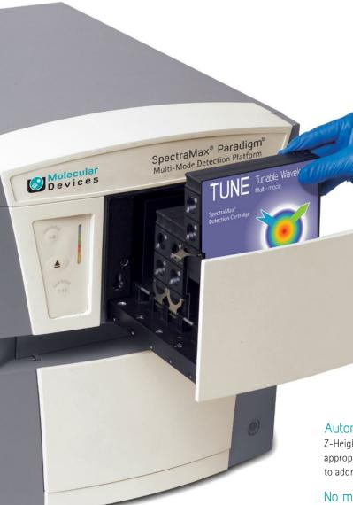
Every SpectraMax® Paradigm® Detection Cartridge starts with an application-optimized excitation energy source either in the form of a long-life, high-powered LED, xenon flash lamp, or high-powered laser. Concentrating the excitation light on the sample through label-specific optics, high levels of sensitivity and performance are reached. All this combined in the detection cartridge creates the ultimate no-compromise multi-mode detection platform.
